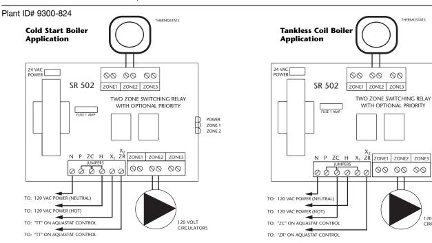
Note: When using Alternative Wiring diagram, the boiler operating control's ZC terminal will see the load of the circulator(s).
